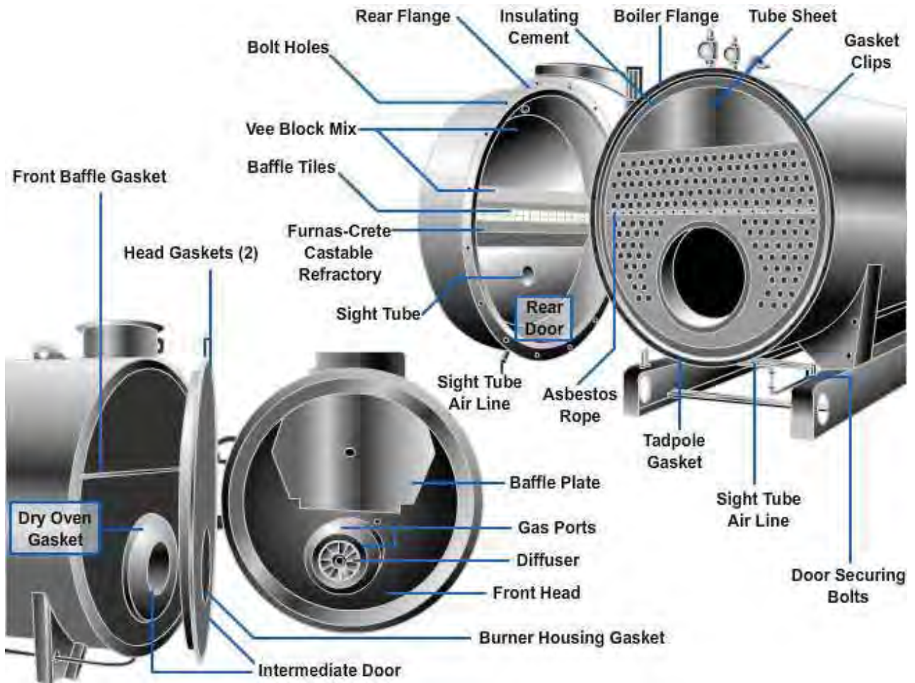
Figure 9-54 - Front and rear doors open on a gas-fired boiler.
