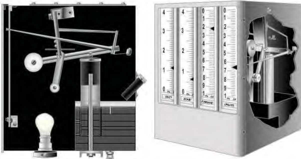
Figure 9-29 - Liquid sealed draft gauge.
