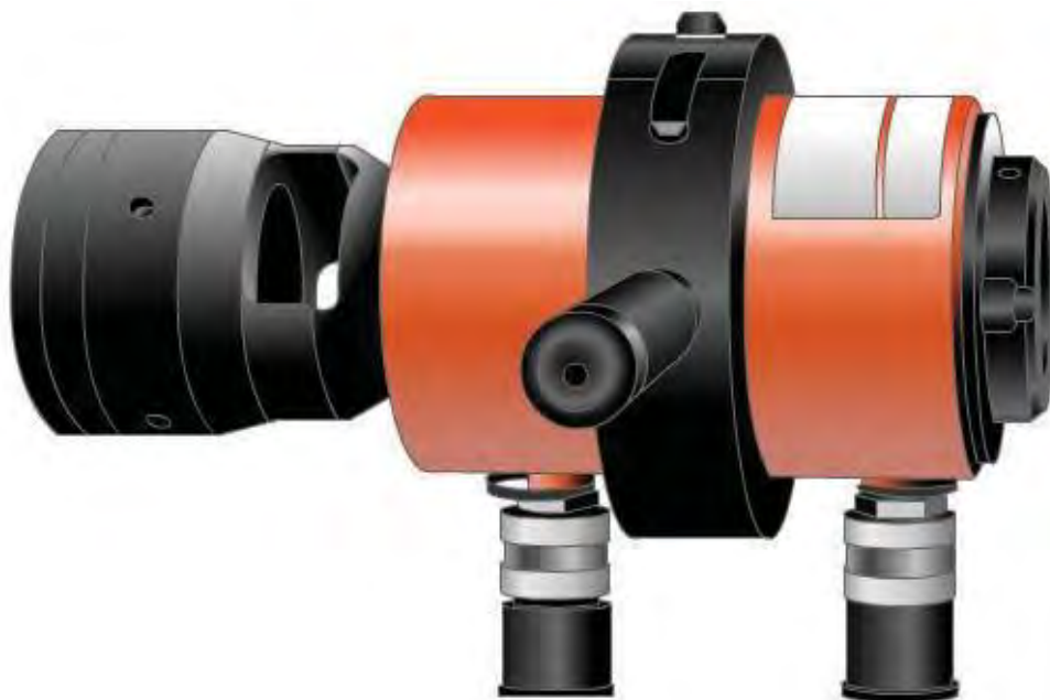
Figure 9-42 -Tube tigger in operation.
