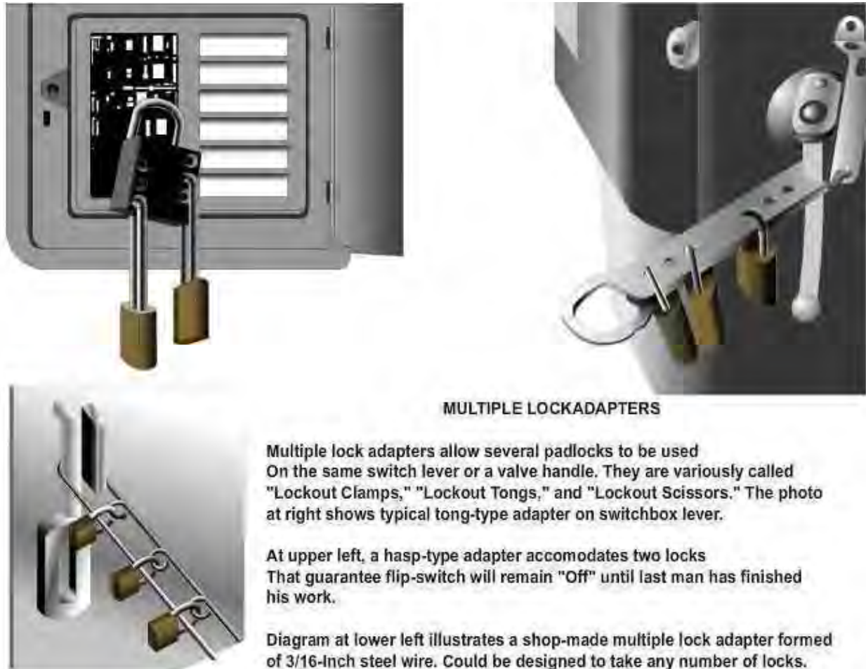
Figure 9-57 - Multiple lock adapters.
